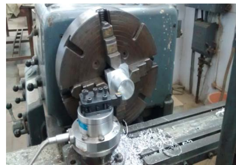
Fig. 3: The workpiece mounted on four jaw chuck
